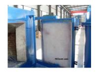
Heavy Duty Incinerator waste feed door, safe and negative pressure operation in combustion chamber.
