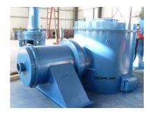
Secondary Chamber & Mix-Combustion Chamber. Residency time 2.0 sec. in post combustion chamber. Virtually smoke and smell free.
