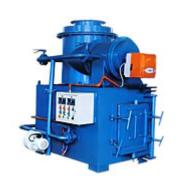
with dual combustion chamber, mix-combustion chamber and smoke filter chamber with refractory lines, and the combustion chamber temperature up to 1200 deg C.
